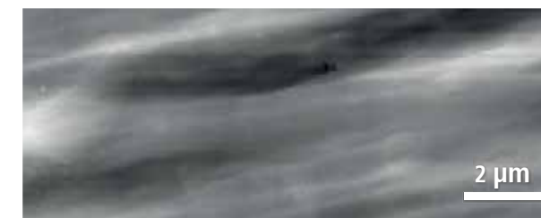
KPFM measurement on cathode composite region of ASS-LIB during CV operation. Surface potential images below are measured while the cell voltages were swept from 2.37 to 2.68 V.
